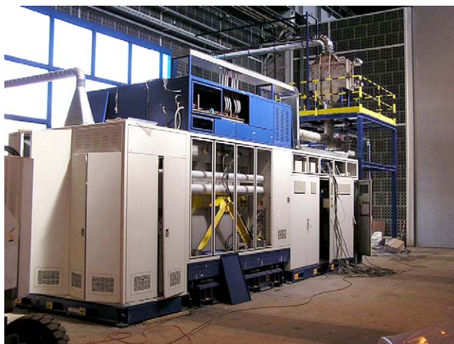
Fig. 1. Picture of the EOS-CHP 100 SOFC Field Unit installed at the GTT factory.
